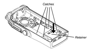
Figure 3-8: Lock Retainer Catches to the Radio's Body
