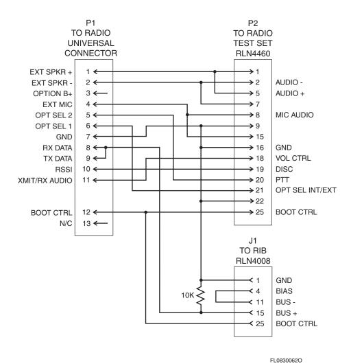
Figure 3-24: Programming/Test Cable Schematic
