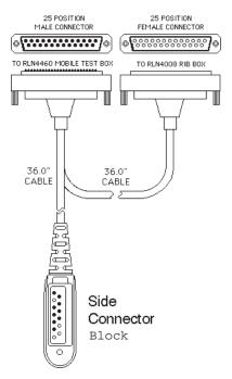
Figure 3-22: Programming/Test Cable AARKN4074
