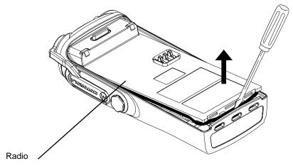
Figure 3-3: Chassis Removal
