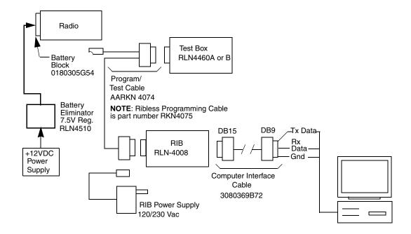
Figure 5-2: CPS Programming Setup
