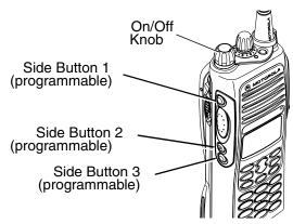
Figure 5-4: HT1550•XLS Radio Side Button Locations
