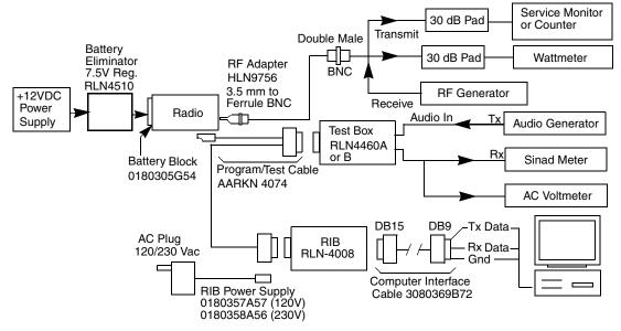
Figure 5-1: Radio Tuning Test Equipment Setup
