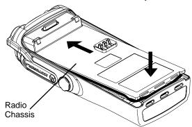
Figure 3-9: Fastening the Chassis
