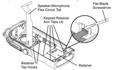
Figure 3-6: Remove Retainer
