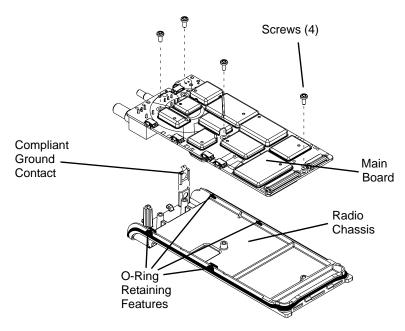
Figure 3-5: Remove Main Board from Chassis
