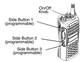
Figure 5-3: Radio Side Button Locations
