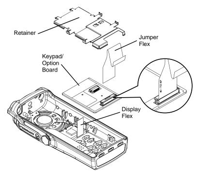
Figure 3-11: Changing Keypad/PassPort Board / Option Boards
