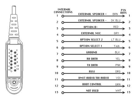
Figure 3-23: Pin Configuration of the Cable Side Connector
