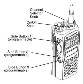
Figure 4-1: Radio Side Button Location
