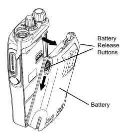
Figure 3-1: Battery Removal
