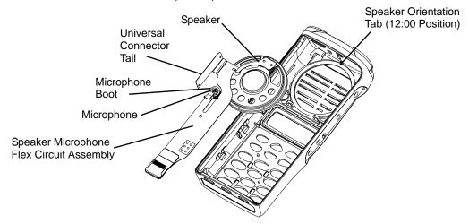
Figure 3-6: Removal Speaker-Microphone Assembly
