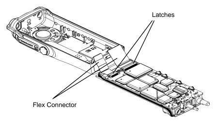
Figure 3-4: Unlatch Flex Connectors
